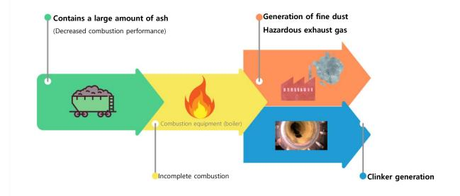
It is <u>the cheapest</u> among the existing energy resources and is widely used worldwide as it is <u>rich in heat</u>. Thermal efficiency is relatively low, air pollution occurs due to incomplete combustion and periodic facility maintenance is required.
